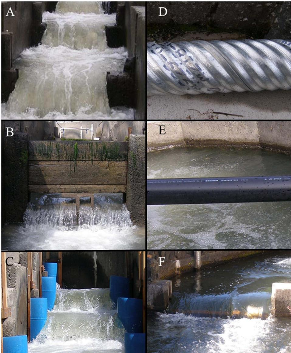
Fig. 1. Experimental treatments tested for passage performance. A indicates Control, B Gap, C Bulkhead, D Culvert, E Tube, F Inverted U. The Gap treatment is shown while the ladder water level has been dropped in order to show the modification that would otherwise be underwater. Image scale varies by treatment and weir boards are 130 cm (A,B,C and F), Culvert (D) is 16.5 cm diameter and Tube (E) is 10 cm diameter.
