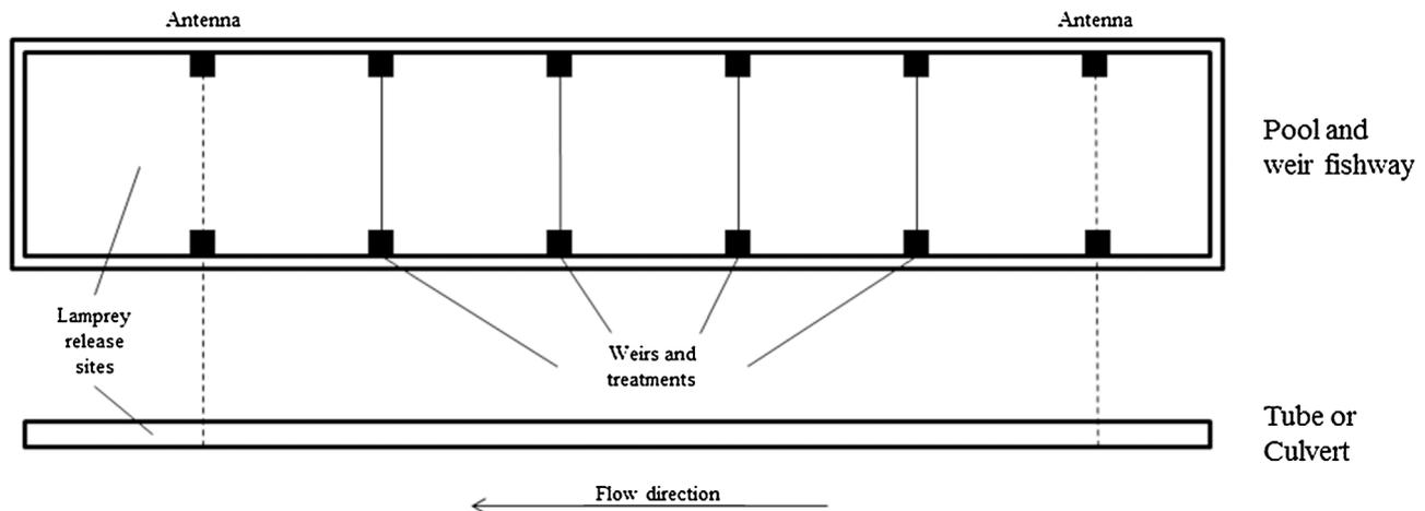
Fig. 2. Plan view of the experimental fishway treatments used to test Pacific Lamprey passage performance. Pool and weir fishway treatments included Control, Gap, Bulkhead.
