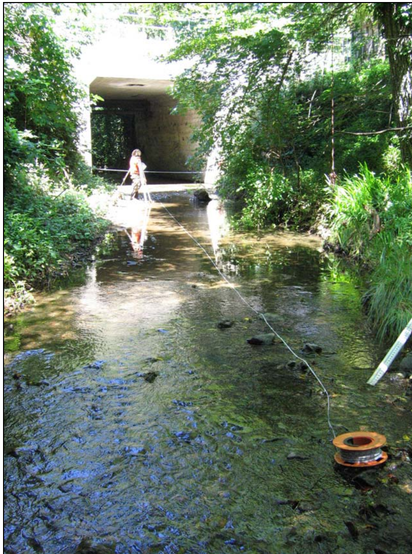
Figure 2. Example of tape locations for measuring cross-section and downstream channel slope, San Anselmo Creek at Fairfax-Bolinas Road.
