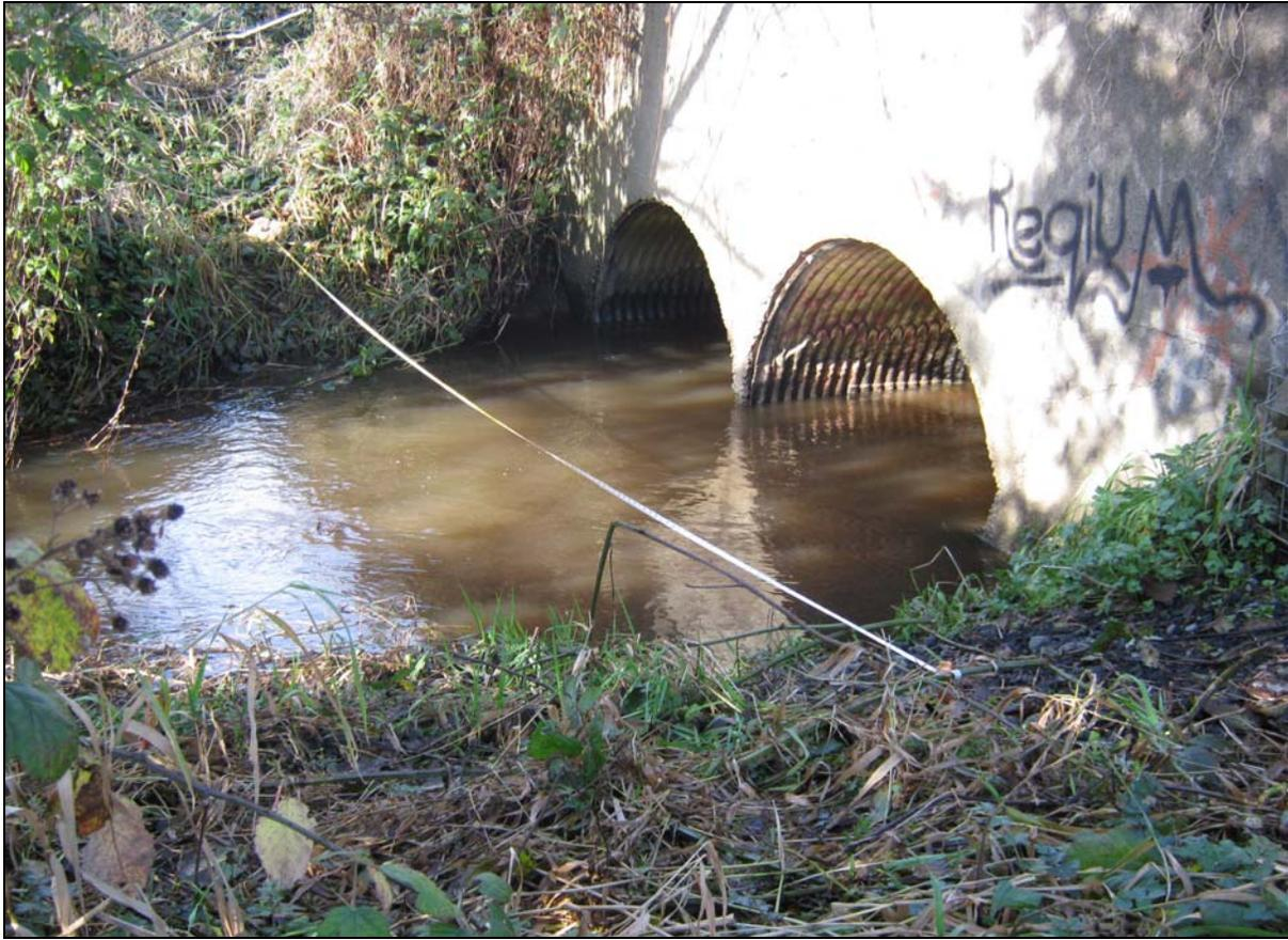
**Figure 2.** Example of tape location for measuring the tail-water cross-section.
