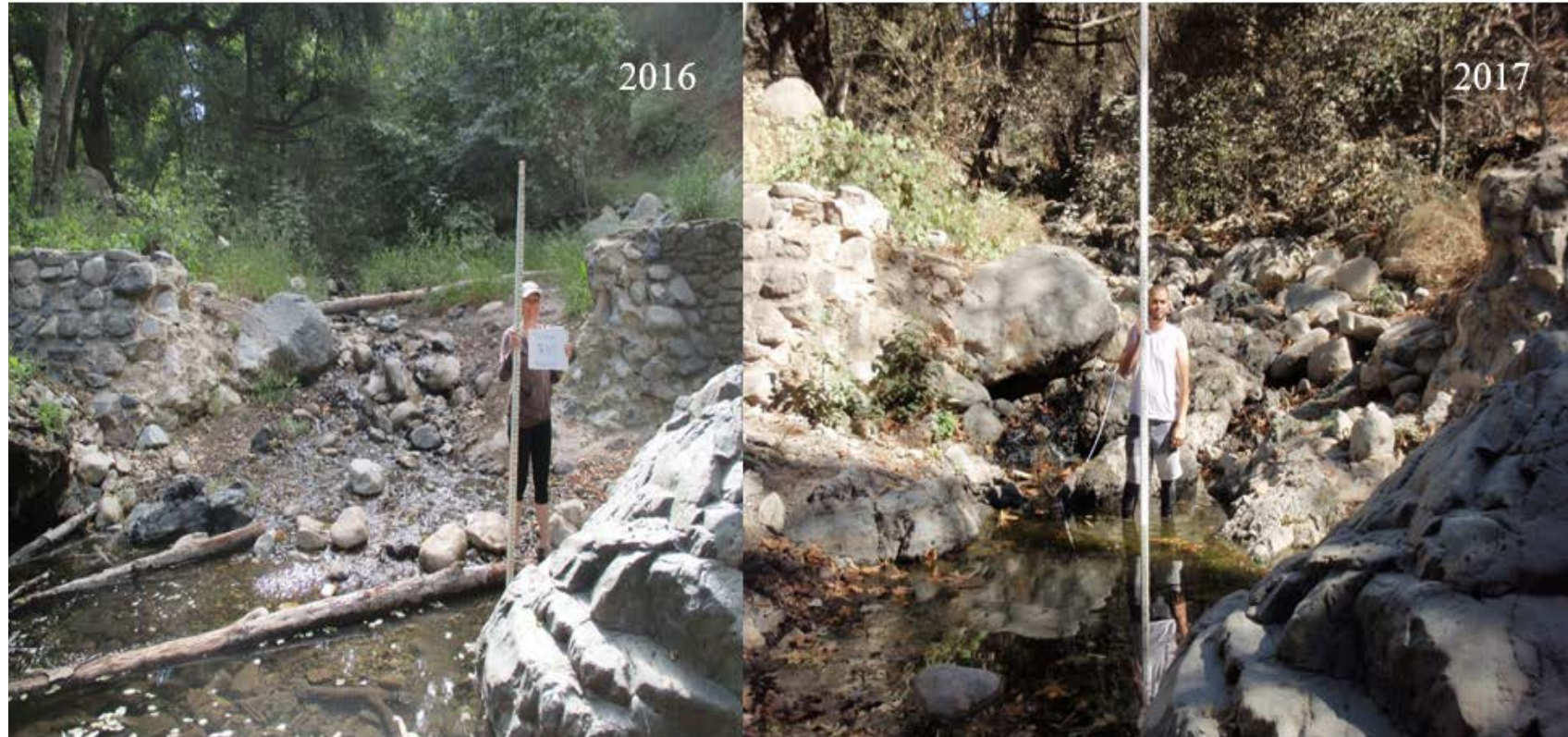
Figure IV-23. Comparison of 2016 vs. 2017 TCFD7 dam removal site in which nearly 2ft of scour was observed in 2017 when compared to 2016.
