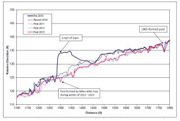
Figure 1. Pre-project, record, and post-project longitudinal thalweg profiles of the Glennbrook Gulch channel, 1,100 to 1,800 feet.
